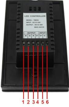
5 and 6: power input, input voltage range: 12-24V, 5 for positive, 6 for negative. 1 ,2,3 and 4: power output, output voltage is 12-24V, Max output current is 8A, 4 for positive, 3 for red led interface, 2 for green led interface, 1 for blue led interface.
